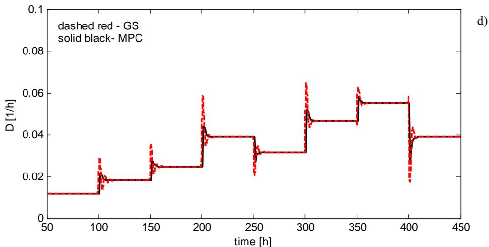
Fig. 6. Simulation results for constant DO setpoint (6.5 mg/l) obtained with the two methods: GS and MPC: a) aeration rate, b) dissolved oxygen, c) substrate, d) dilution rate
