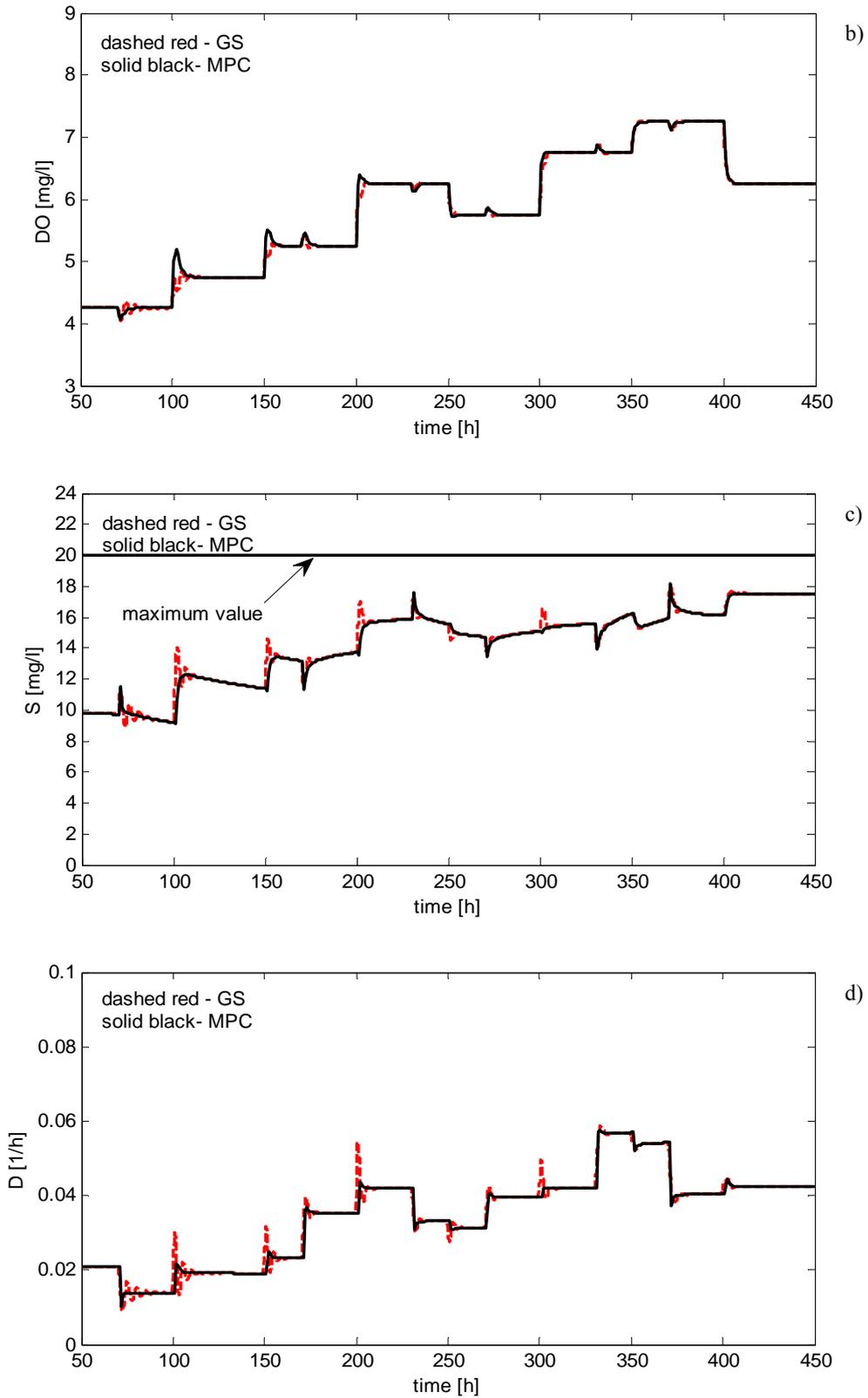
Fig. 8. Simulation results for variable DO setpoint and substrate concentration in influent ( $S_m$ ) obtained with the two methods: GS and MPC: a) influent substrate concentration variation, b) dissolved oxygen, c) substrate, d) dilution rate
