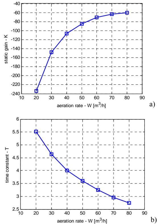
Fig. 4. Parameters values of the linearized model of the wastewater treatment process: a) static gain; b) time constant
