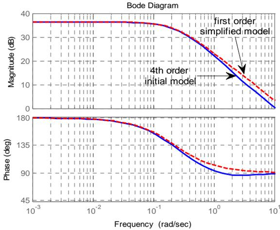
Fig. 3. Modal analysis of the linearized dynamics between  $D$  and  $DO$
