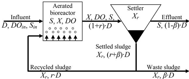
Fig. 1. Diagram of the activated sludge process
