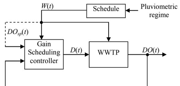
Fig. 2. Gain scheduling scheme for dissolved oxygen control
