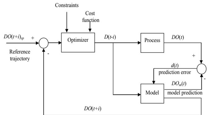
Fig. 5. MPC block diagram
