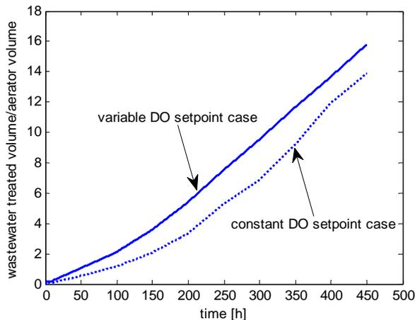
Fig. 9. Wastewater treatment process efficiency (the amount of treated wastewater with the same electrical power consumption) with gain scheduling method for constant DO setpoint case (dotted line) and variable DO setpoint case (solid line)
